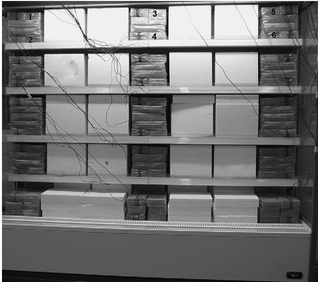
Fig. 3. Temperature test inside display case.
